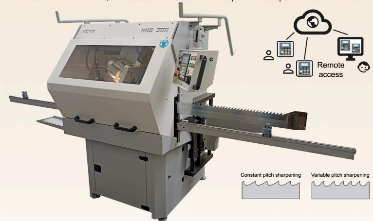
The NBS 300-G is equipped by transverse axis and therefore trapezoidal or alternately slanted teeth can be sharpened. Another advantage of the machine is the servo-controlled feeding finger, which ensures a faster cycle run, since it starts to feed as soon as the grinding wheel moves back.
